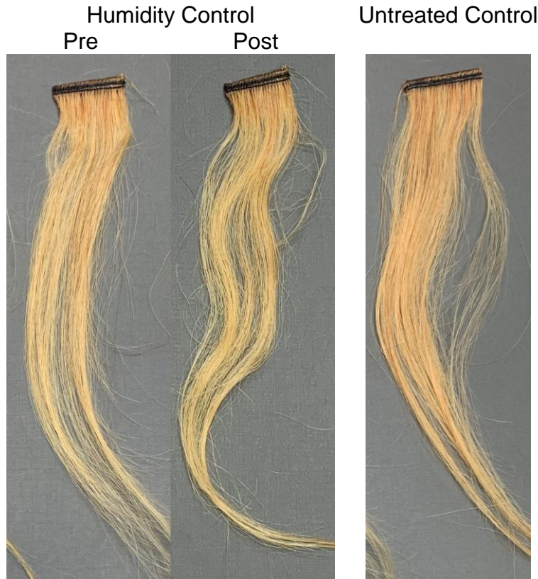
Figure 2: Pre-humidity Exposure and Post 30-minutes Humidity Exposure of Control Bleached Hair Swatches
