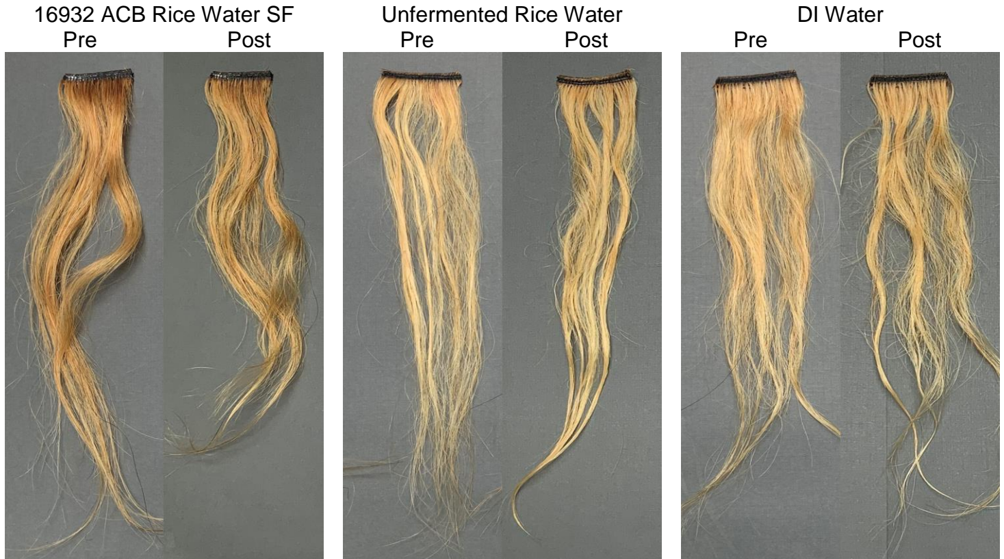
Figure 1: Pre-humidity Exposure and Post 30-minutes Humidity Exposure of Treated Bleached Hair Swatches
