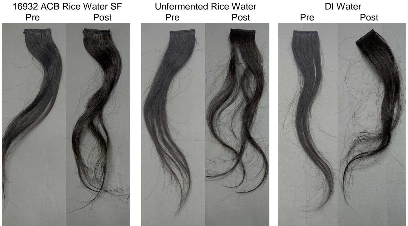
Figure 3: Pre-humidity Exposure and Post 30-minutes Humidity Exposure of Treated Virgin Hair Swatches
